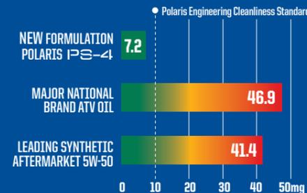
ASTM D6335. In 3rd party against 9 competitive products Polaris PS-4 had less than half the deposits compared to the next closest product. No other tested products met Polaris Engineering standards for deposit cleanliness.
